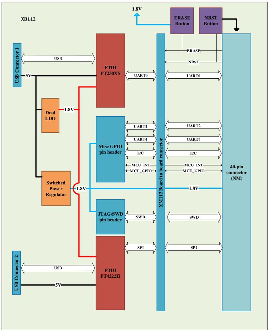
Figure 1 The EVK block diagram.
