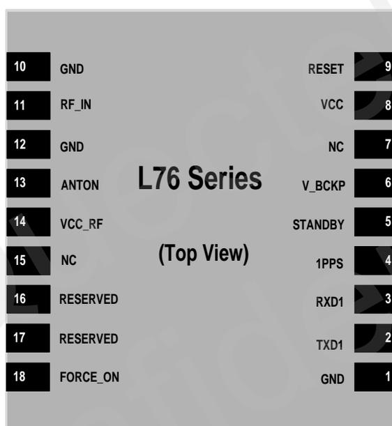
Figure 2: Pin Assignment
