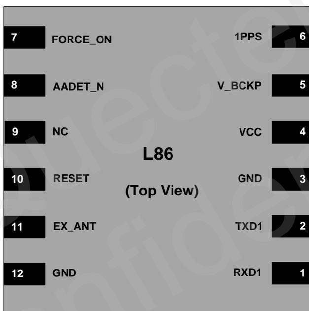
Figure 2: Pin Assignment
