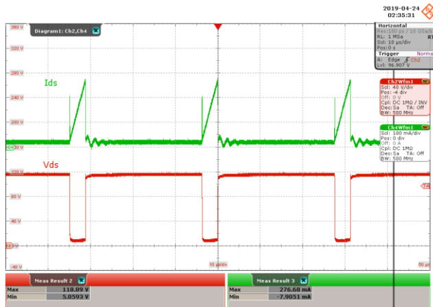
Figure 14 – Drain Voltage and Current Waveforms. 85 VAC, 120 mA Output. Upper: I DRAIN , 100 mA / div. Lower: V DRAIN , 40 V, 10 μs / div. I MAX = 276.7 mA, V MAX = 118.9 V.
