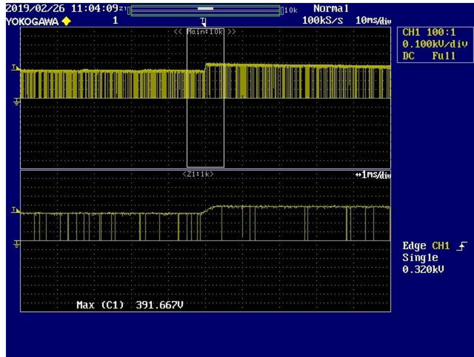
Figure 40 – Drain Voltage, 230 VAC, Full Load.
