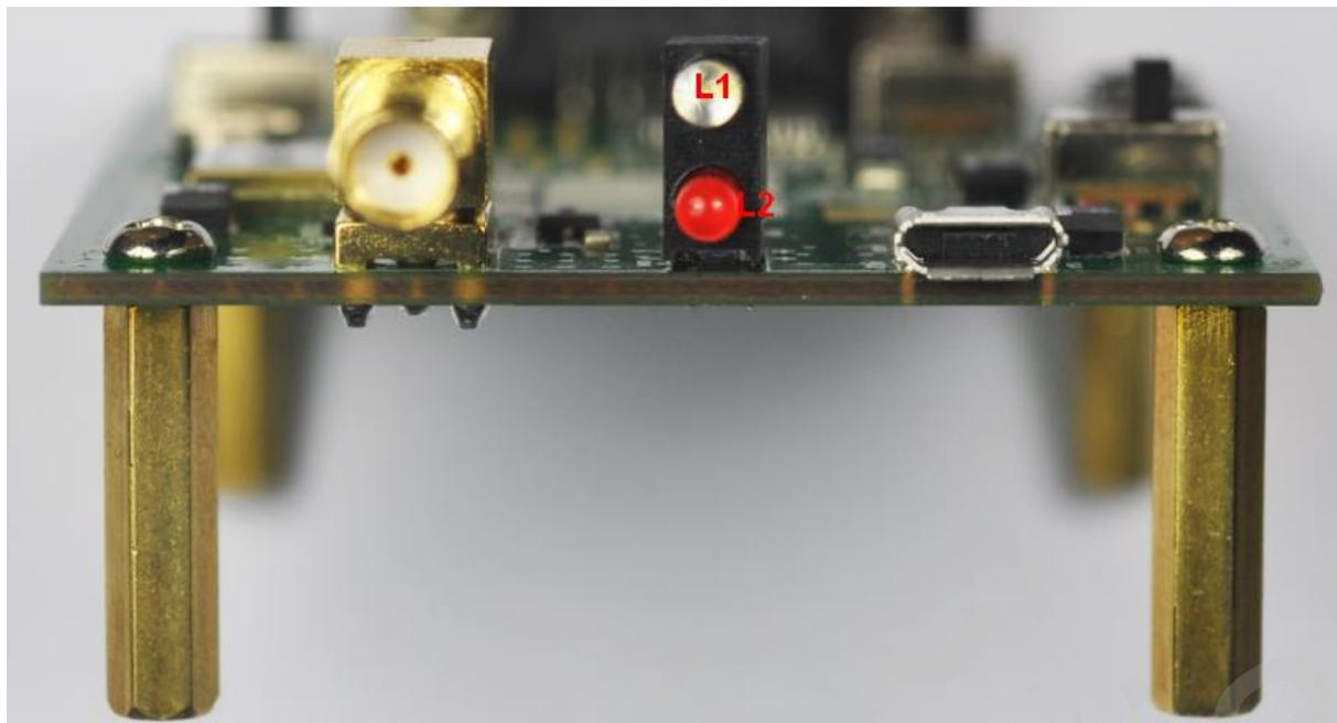
Figure 9: Operating Status LEDs
