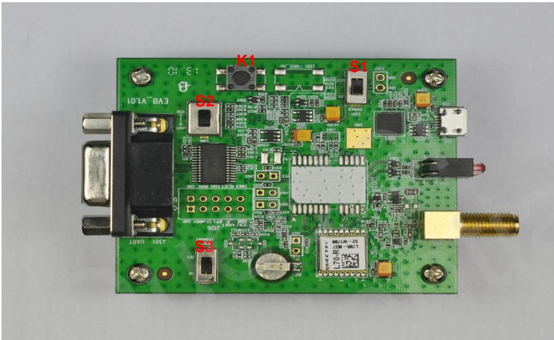
Figure 8: Switches and Buttons
