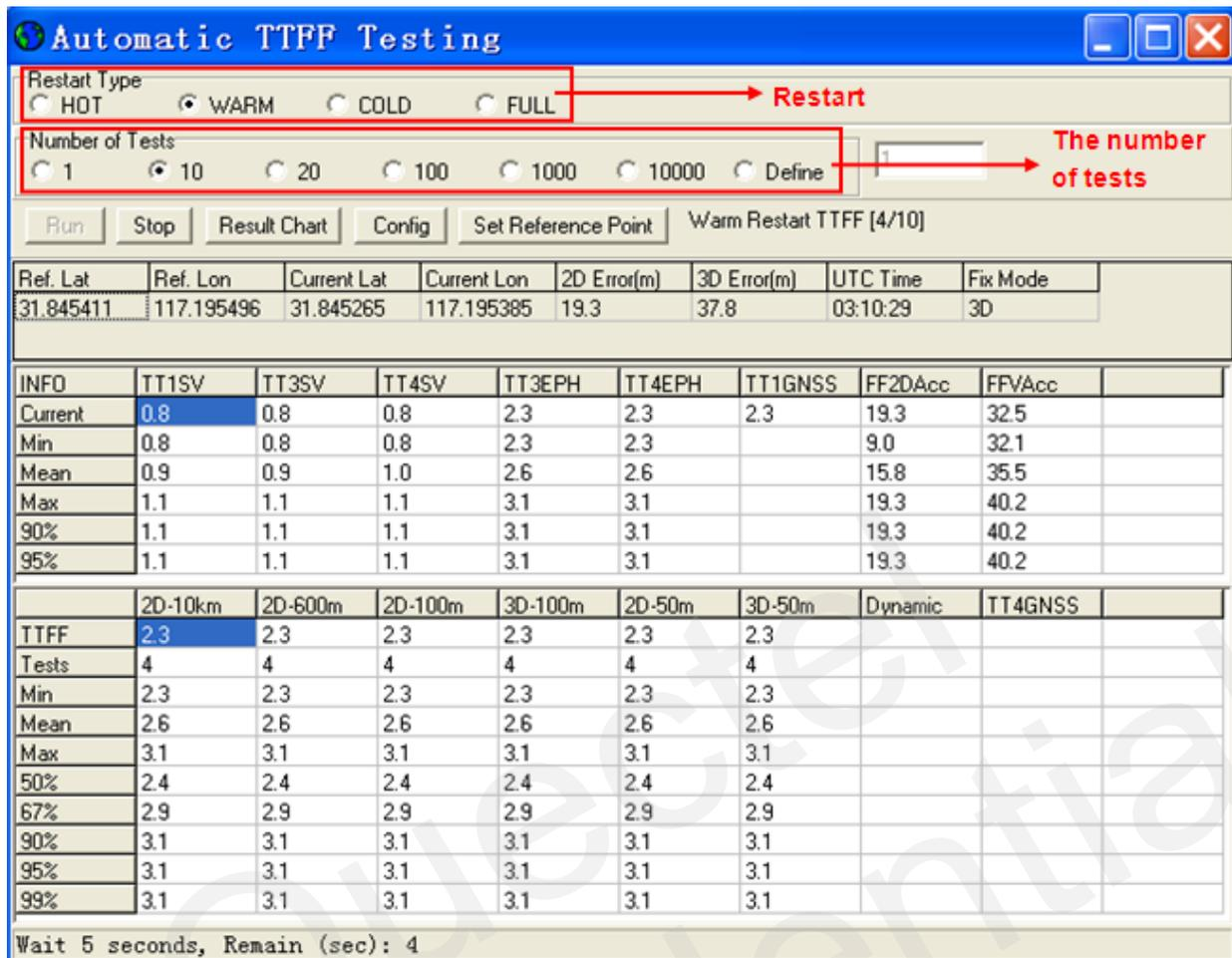
Figure 14: Static TTFF Testing
