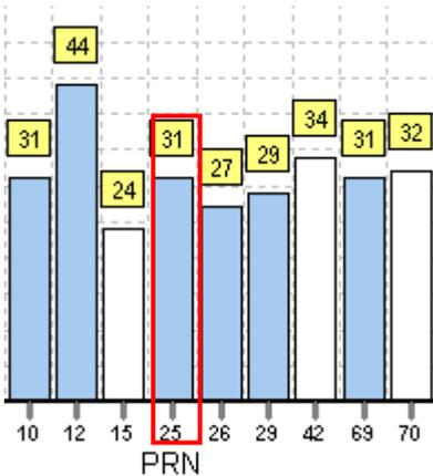
The CNR of PRN 25 is 31dB/Hz. Light blue column means the navigation data of this satellite is in use.
