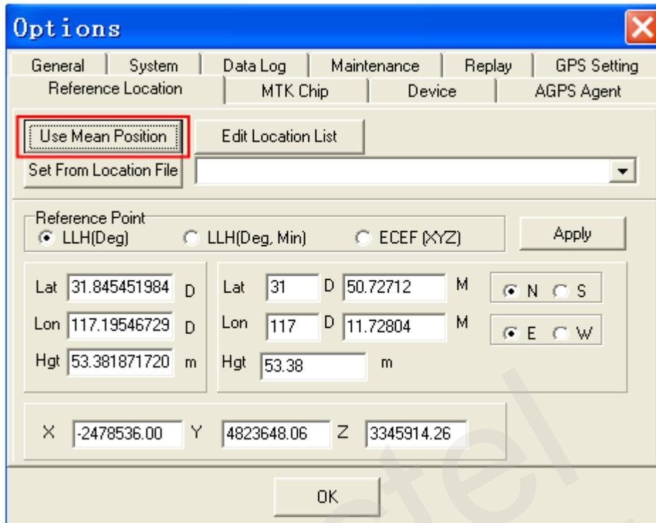
**Figure 15: Static TTFF Testing Configuration Options**
