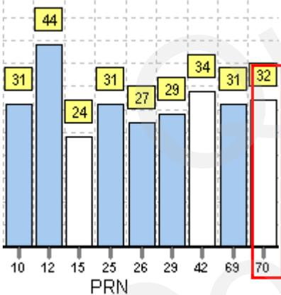
The CNR of PRN 70 is 32dB/Hz. White column means the navigation data of this satellite is not in use. The range of GLONASS SVID is 65-96.
