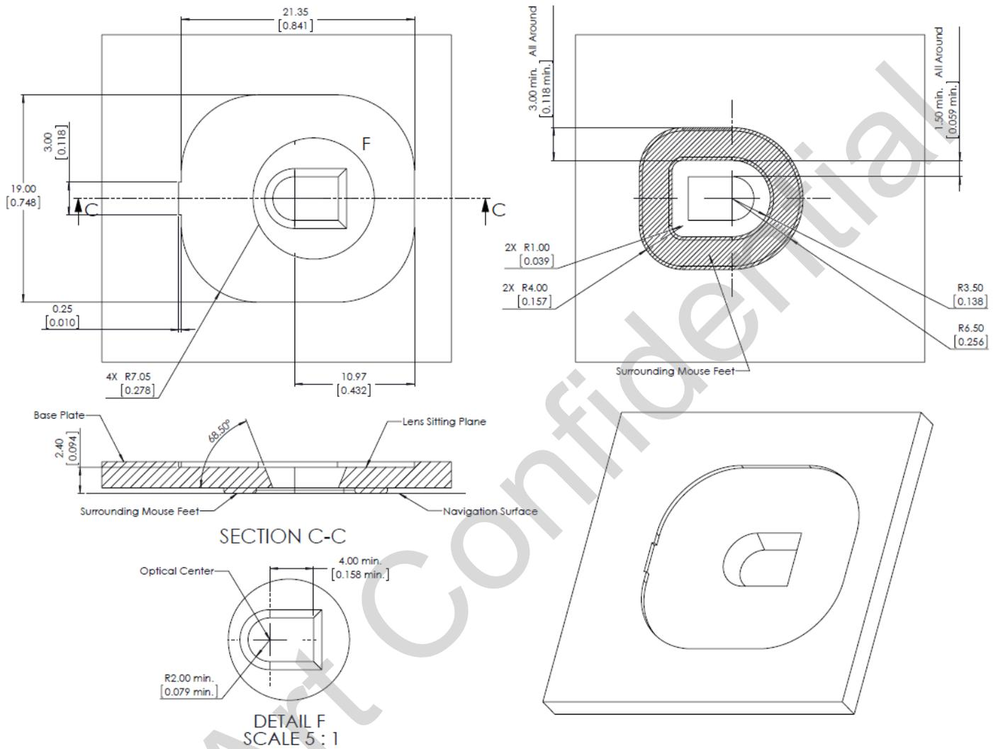
Figure 8. Recommended Base Plate Design
