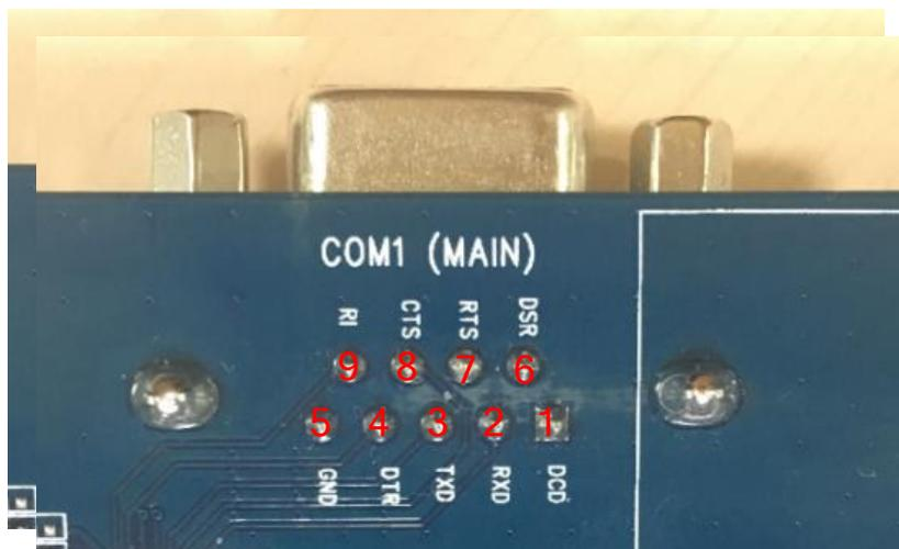
**Figure 25: Pin Assignment of J401**
