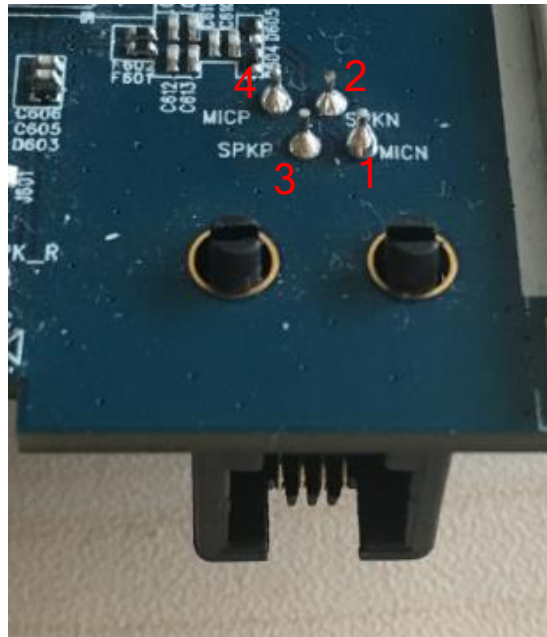
Figure 18: Pin Assignment of Handset Connector J602
