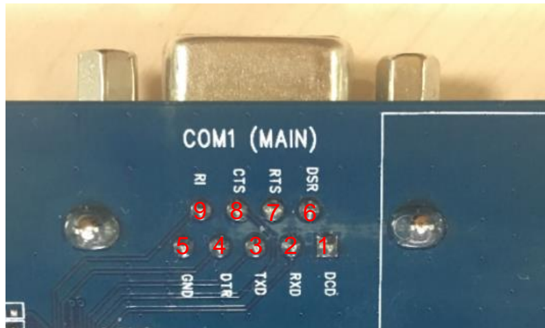
Figure 25: Pin Assignment of UART Connector J401
