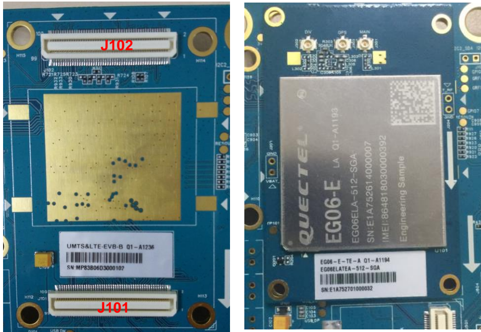
Figure 10: Connection between TE-A and EVB
