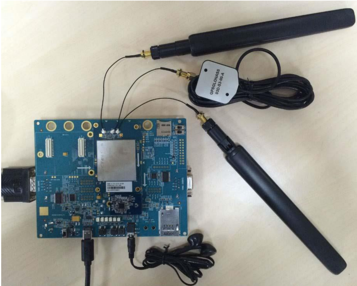
Figure 6: UMTS&LTE EVB R2.0 and Accessories Assembly
