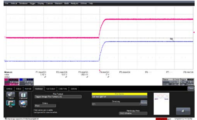
Figure 37 – Output Voltage and Current Waveforms. 265 VAC Input. Upper: 5 V, 2 V / div. Middle: I_{OUT} , 1 A / div. Lower: 12 V, 5 V, 1.6 ms / div.
