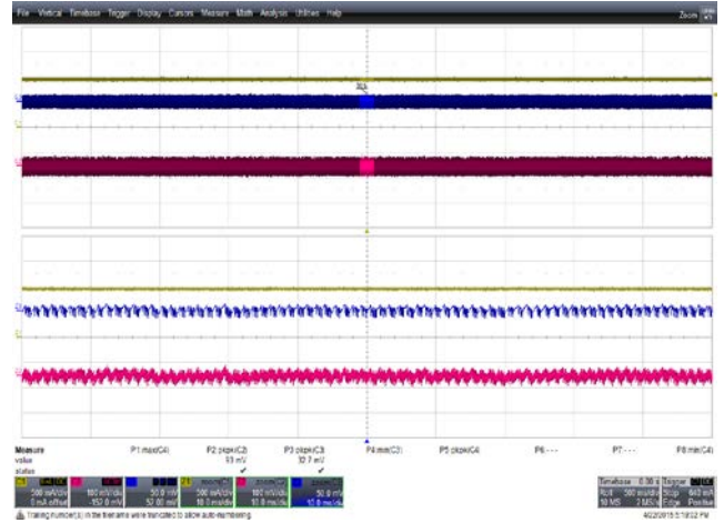
Figure 49 – Output Ripple Voltage Waveforms. 265 VAC Input. 1.0 A on 12 V. 5 V PK : 33 mV, 12 V PK : 93 mV. Upper: 5 V, 50 mV / div. Lower: 12 V, 100 mV /, 500 ms, 20 ms / div.
