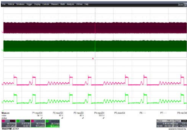
Figure 34 – SR FET Voltage Waveforms. 265 VAC Input, Full Load. (83 V MAX for 12 V, 34 V MAX for 5 V.) Lower: 12 V, 50 V / div. Upper: 5 V, 20 V / , 6.4 ms, 10 μs / div.
