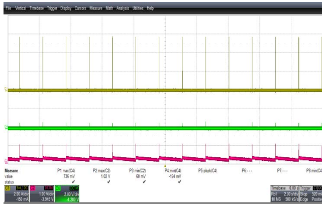
Figure 40 – Output Voltage and Current Waveforms. 85 VAC Input. Upper: I_{OUT} , 2 A / div. Middle: 12 V, 2 V / div. Lower: 5 V, 1 V, 2 s / div.
