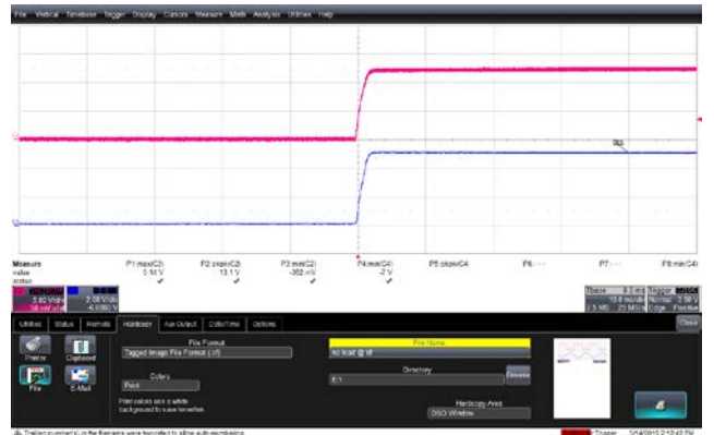
Figure 39 – Output Voltage and Current Waveforms. 265 VAC Input. Upper: 5 V, 2 V / div. Middle: I_{OUT} , 1 A / div. Lower: 12 V, 5 V, 1.6 ms / div.
