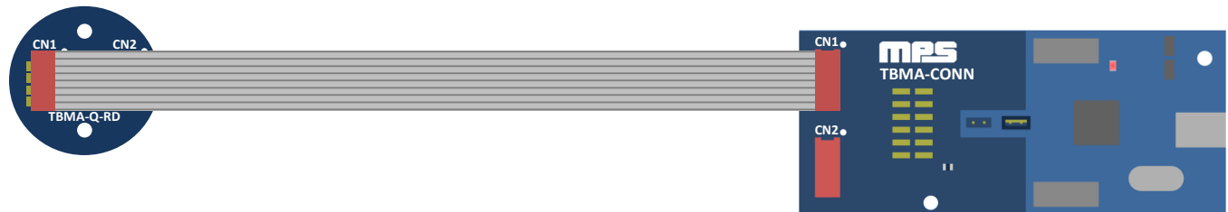
Figure 16: Connect TBMA-RD to TBMA-CONN Board
